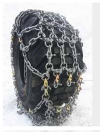
7. Connect the mesh. Use the additionallinks enclosed if necessary. Usually it's easiest to connect the outer part of thetag chain first
