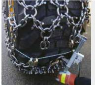
**6.** Use the Olofsfors installation tool to pull the ends together
