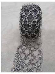
**5.** Check the center of the chain patternfollows the centre of the tire pattern.
