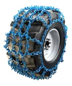
**Olofsfors PRO-Grip SF™**, is our latest model. With its transversely arranged, forged, and studded grousers, both grip and service life are increased greatly.
