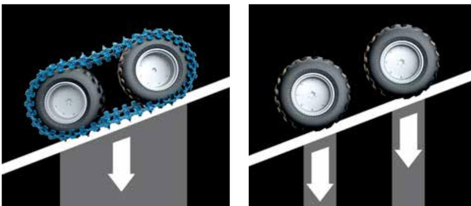
*With tracks, the machine will have a larger contact surface and the centre of gravity is distributed over a greater area.*
