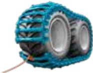
2. When the track is on the bogie make sure that the ends are at one end of the bogie.
