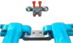
**8.** Tighten the track until you can install the track lock.
