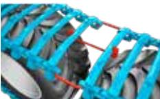
5. Mount the installation tool on the cross members from below. Make sure that it is in the middle. **NOTE:** If the tires are new, it helps mount significantly, if you moistens them. It may also be needed to help push up the track from the short edge towards the top.
