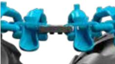
**11.** Take out the tool. The proper tensioning of the track is when slack between tires is max. 50 mm.
