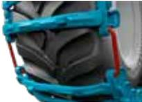
3. Mount the two clamps from the outside into the link hooks.
